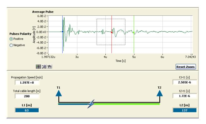
PD was located at 63 m from the measurement point
