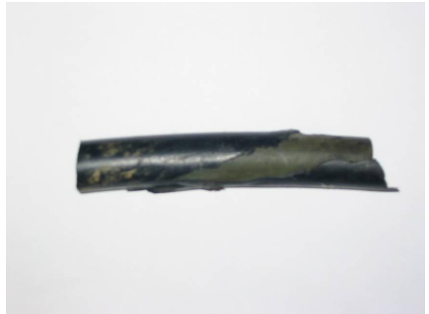
Chemical Exposure (Causes cable degradation)
