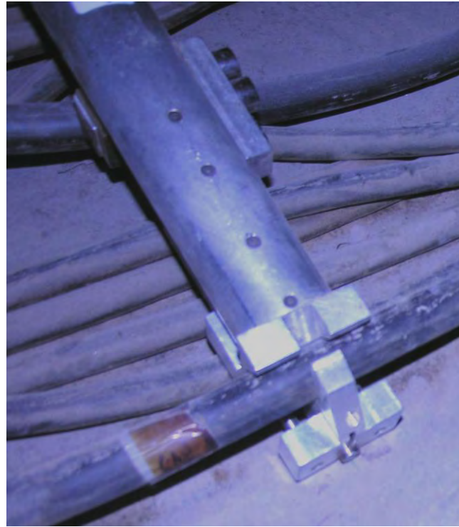
The Indenter Tool in a cable tray as used in the field
