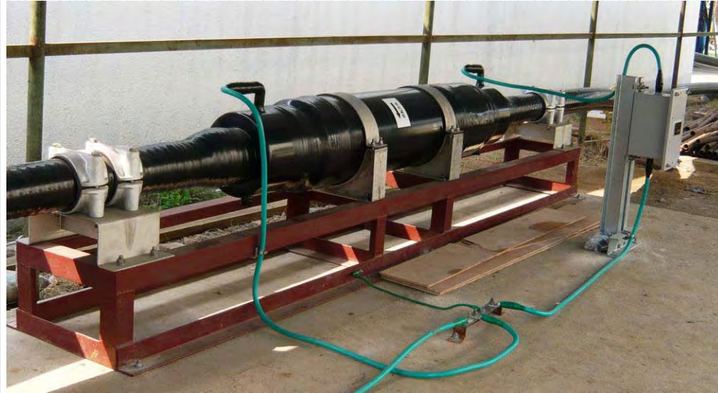
Prefabricated Type Joint
